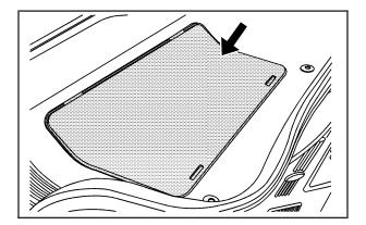
The access panel for the passenger compartment air filter is located under the hood near the windshield, on the passenger's side of the vehicle.
